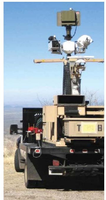
Telephonics' MSS system on Kitt Peak, AZ during 18 km radar vehicle detection test
