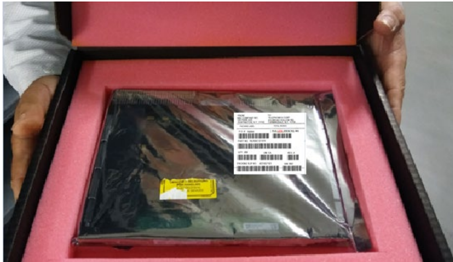
Figure 2 - Sample ESD Protective Wrapping of Unit (with Label on Wrapping) Contained in Outer ESD Protective Box with Inner ESD Protective Lining
